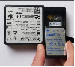
**Step 2:** Ensure the blue arrow on the battery and the blue arrow in the compartment match.
