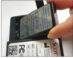
**Step 3:** With the battery label facing up, set the battery into the compartment at an angle on top of the pull ribbon. **DO NOT** force the battery down flat on top of the battery contacts.
