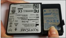
**Step 4:** Firmly press the other end of the battery down into the compartment. The battery will now sit flat in the battery compartment on top of the pull ribbon and the device will power on.
