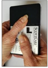
**Step 1:** Remove the battery cover by pressing down on the lines and pushing away from the device.
