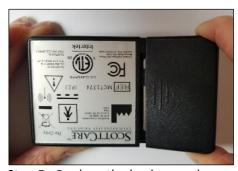
**Step 5:** Replace the back cover by inserting it at an angle to align the tab with the device. Once aligned, press down and push close to close the battery cover.
